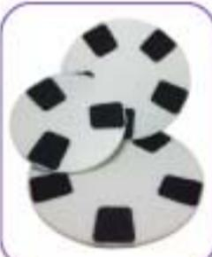
To be used as segment-holder plate for any kind of floor shining machine. With 3 or 5 velcro supports in both sides. It is fitted to the machine by a standard floor pad interposed between the plate and the driving plate of the machine, or also directly attached to the rubber cover of the driving plate.
